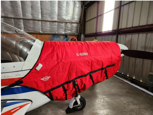
ZLIN 142C Insulated Engine Cover
