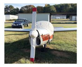
Aerotechnik L-13 Vivat Motorglider Prop/Spinner & Canopy Covers
