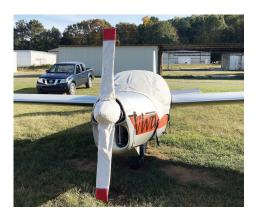
Aerotechnik L-13 Vivat Motorglider Prop/Spinner & Canopy Covers
