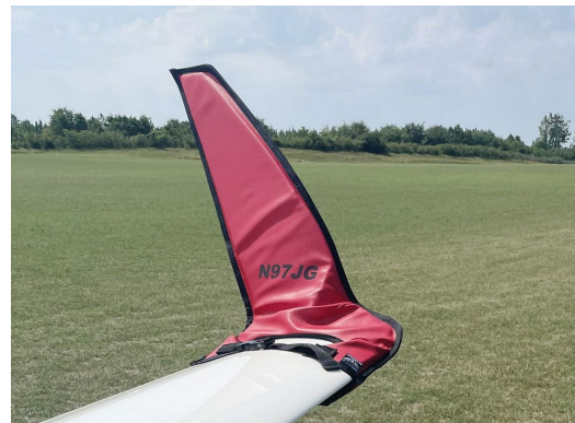
Schempp-Hirth Ventus-2B winglet/wingtip pads
