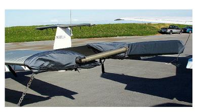
End Cap Covers are used when wing are in folded position.
