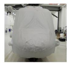
Sikorsky S-92 Windshield/Nose Cover, test fit cover
