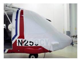
Sikorsky S-92 Windshield/Nose Cover, test fit cover
