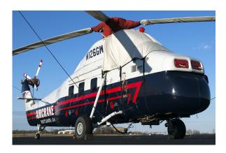
Sikorsky S58T Canopy, Rotor Hub, Blade, Tail Rotor Covers, Engine Plugs, Blade Tie-Downs
