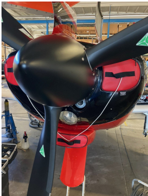
ENGINE PLUGS PREVENT BIRD NEST FOD. Piper Saratoga Engine Cowling Bird's Nest Siai Marchetti SF260 Engine Plugs
