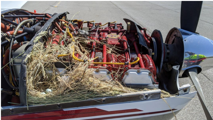
ENGINE PLUGS PREVENT BIRD NEST FOD. Piper Saratoga Engine Cowling Bird's Nest Siai Marchetti SF260 Engine Plugs
