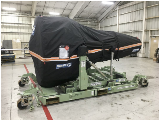
CFM56-5B Off Link Cover, fully enclosed
