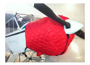
Piper Super Cub Insulated Engine Cover
