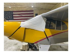
Piper J5A Windshield/Skylight Cover, test fit
