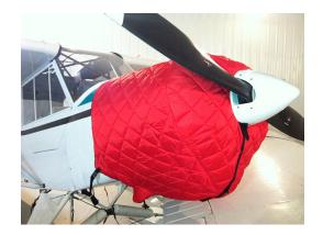
Piper Super Cub Insulated Engine Cover
