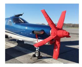
Socata TBM Insulated 5-Blade Prop/Spinner Cover
