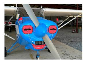
Piper PA-22-150 Engine Inlet Plugs (set of 3)
