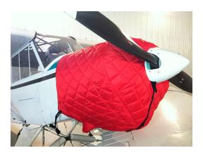
Piper Super Cub Insulated Engine Cover
