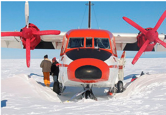
Casa 212 Insulated Engine & Propellor/Spinner Covers
