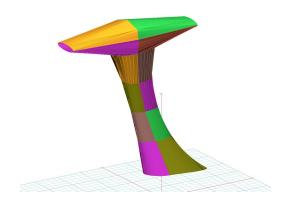
Autogyro Calidus Rotor Mast Cover, 3D model
