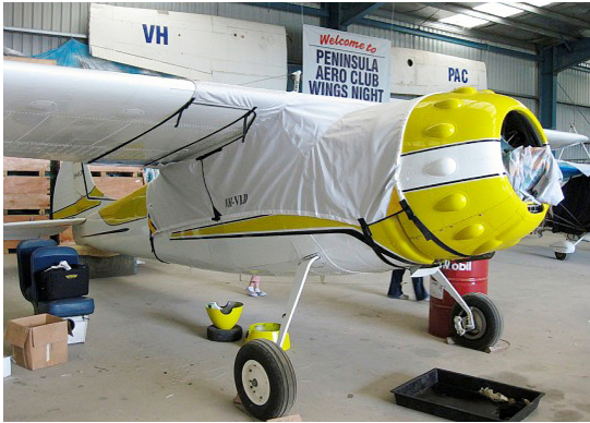
Cessna 195 Canopy Cover, extended forward and over gas caps Cessna 195 Canopy Cover, over-top, 24" fwd ext to cover cowl ring gap, gas cap ext.
