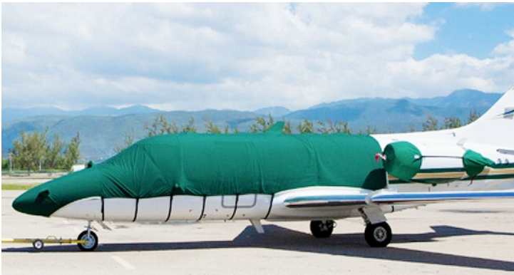
Raytheon Beechjet 400 Fuselage/Nose Cover, Engine Covers
