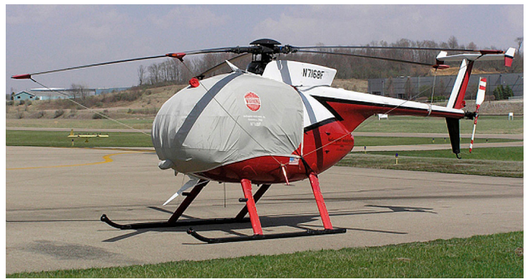
Hughes 500D Bubble Cover with Wire Strike detail and Blade Tie-downs
