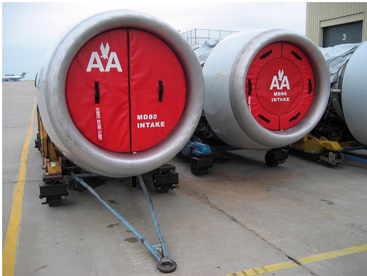
MD-80 JT8D Intake Plugs, Solid Foam folding type& Mesh Center folding type PW JT8D Off-Link Engine Storage Cover w/ Nose Cowl & TR's, "Rain Cap" style
