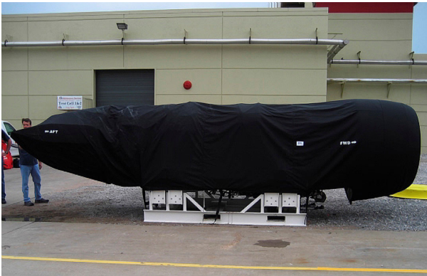
MD-80 JT8D Intake Plugs, Solid Foam folding type& Mesh Center folding type PW JT8D Off-Link Engine Storage Cover w/ Nose Cowl & TR's, "Rain Cap" style
