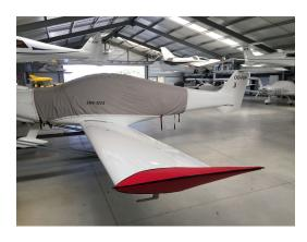
Dynaero MCR.4 Pickup Canopy Cover, Wingtip Pads
