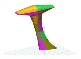
Autogyro Calidus Rotor Mast Cover, 3D model
