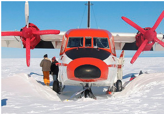
Casa 212 Insulated Engine & Propellor/Spinner Covers
