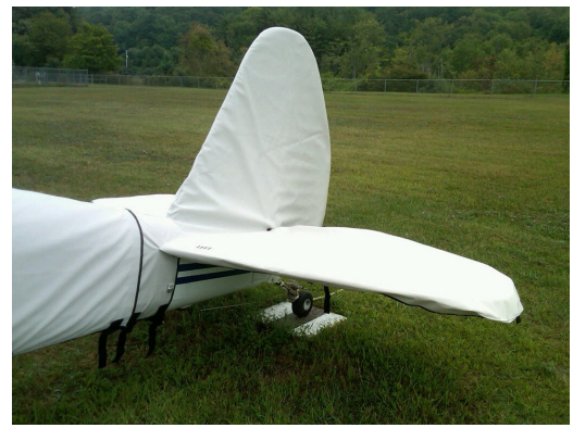
Luscombe Empennage Cover, two-piece design
