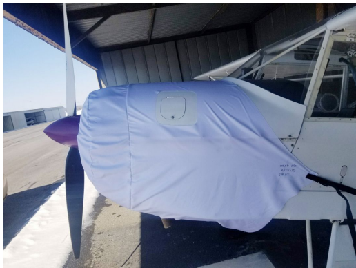
Kitfox Engine Cover, "Radial Cowl" type, test fit
