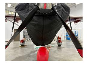
Quest Aircraft Kodiak Insulated Propellor/Spinner Cover, Quest Kodiak Insulated Engine Cover w/Prop Ties, Nose Wheel Cover 4 Blade (padded)
