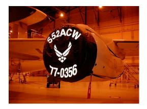
Intake/Exhaust Covers, soft type, TF-33 Engines
