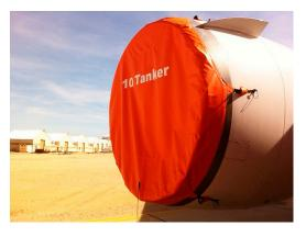
DC-10-30 Intake Cover (CF650C2 Engine)
