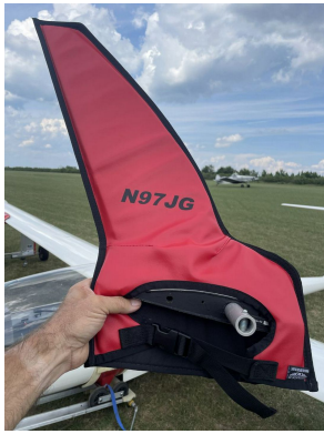
Schempp-Hirth Ventus-2B winglet/wingtip pads
