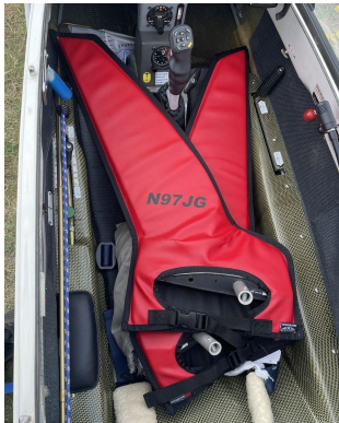
Schempp-Hirth Ventus-2B winglet/wingtip pads
