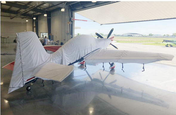
Gamebird GB-1 Extended Canopy/Engine Cover, 3D model Gamebird GB-1 Extended Canopy/Engine, Wing & Empennage Covers (test fit covers)
