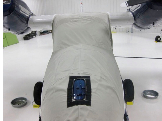
Grumman Widgeon Cockpit/Nose Cover, tie-down cleat detail
