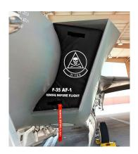
Joint Strike Fighter F-35 Engine Intake PLUG ASSY
