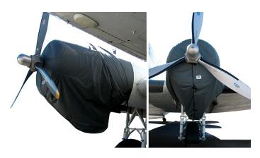
DC3 Engine Covers are custom made for various engine mod's.
