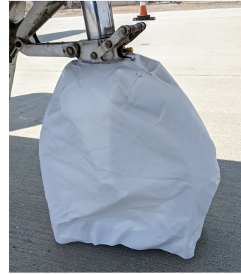
CJ1 Nose Gear Tire Cover, test fit
