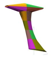
Autogyro Calidus Rotor Mast Cover, 3D model
