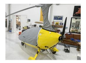
Autogyro Calidus Gyrocopter Canopy/Nose & Rotor Hub/Mast Cover
