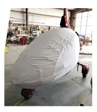
Cavalon Gyrocopter Bubble Cover, test fit cover
