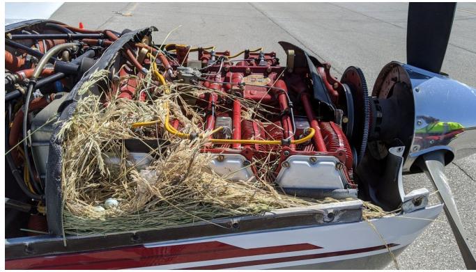
Britten-Norman Islander Engine Plugs ENGINE PLUGS PREVENT BIRD NEST FOD. Piper Saratoga Engine Cowling Bird's Nest
