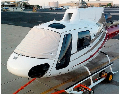
AS350 Windshield Cover, pinches in door jambs
