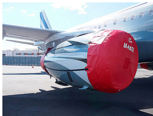
Airbus A319 Intake/Exhaust Covers set, IAE V2500
