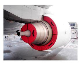
Boeing 737 Bypass and Exhaust Plugs
