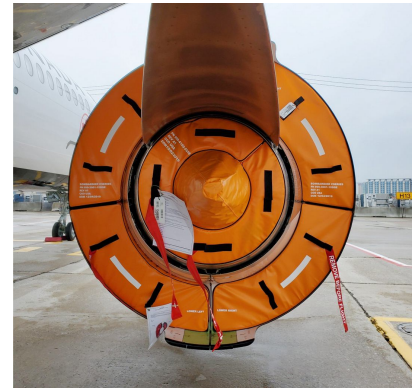
Airbus A320 Exhaust & Bypass Vent Plugs
