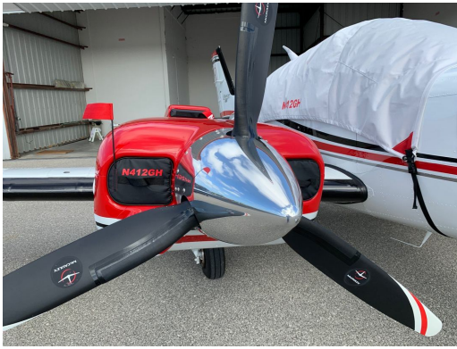
Beech Baron G58 Engine Inlet Plugs
