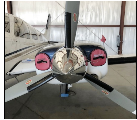
Beech Baron 58P Engine Inlet Plugs
