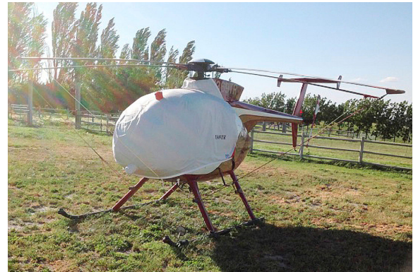
MD500D Bubble Cover with Intake Add-On
