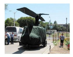
Forward Cabin Nose & Mid-Cabin/Engine Cover (extended to cross tubes)
