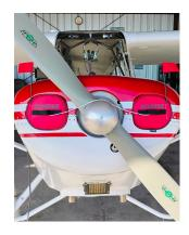
Aeronca 7AC Engine Inlet Plugs
